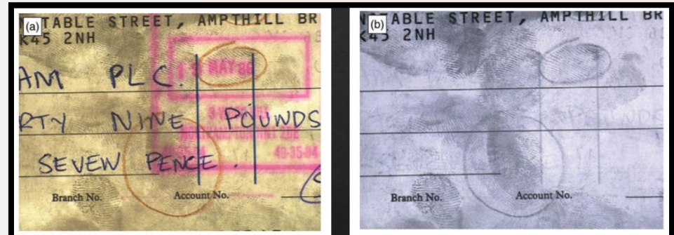
Figure 6.33 Images of fingerprint developed using physical developer on a patterned background: (a) imaged under tungsten illumination and (b) imaged under tungsten illumination using an infrared long-pass filter (Schott glass RG830).
