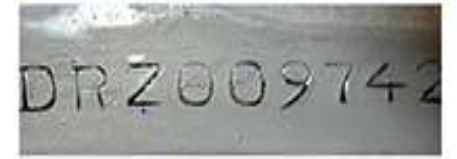
Image 4.1—Front view of the hita truck. Image 4.2—The location of the original chassis number has been ground away and a new number stamped on top. Image 4.3-4.4—The restored chassis number.
