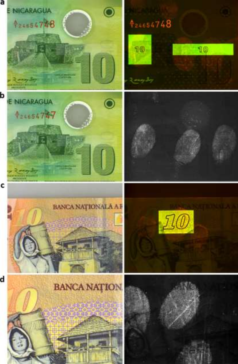
Figure 8: Seven-day-old latent fingerprints on polymer banknotes
