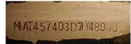
Image 3.1—Front view of the left truck. Image 3.2—The location of the original chassis number has been deeply ground away and stamped on top with a new number. Image 3.3—Restored chassis number. Image 3.4—The original unstamped engine number.
